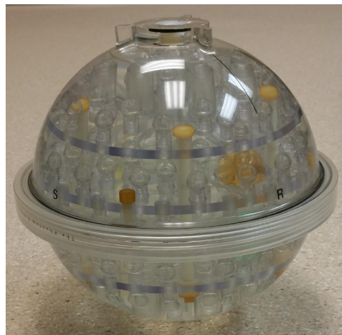
Figure 1. The ADNI phantom used in this work. The phantom is a 20 cm spherical shell that has 160 spherical fiducials (1.0 cm or 1.5 cm in diameters) with known positions.
